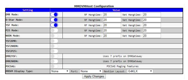
Here you are able to choose what modes are active. No other modes then shown are currently available. Please note, that the modes to use as 'transcoding' like YSF2DMR will not work for now. You can test with DMR2NXDN for example. As you can see no display is selected, we display in a different way. And apply to save.
