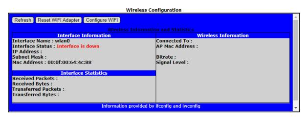
To add your wifi, simply click on configure wifi. Make sure the wifi-dongle is connected to the radio, this screen will only be shown when this dongle is available.
